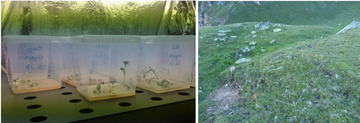
Figure 2.7 Laboratory experiments (left) and vegetation plots (right) to test bacteria-assisted vegetation cover to stabilise slopes in areas of glacier retreat above the timber line.
