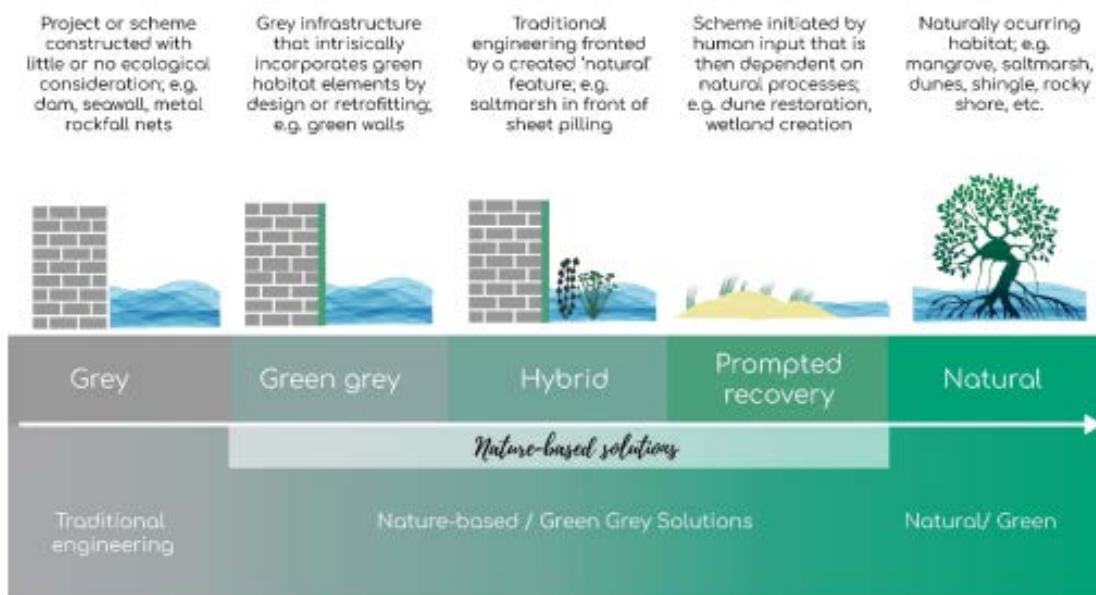
Figure 2: The green-grey continuum of grey to green infrastructure approaches (adapted from: Naylor et al., 2017. Sources: Mangrove by ruliani, wall by AlyaNafisa, dune by Daan, sea plant by Agne Alesiute, Seaweed by Vladimir Belochkin from the Noun Project; Design: Juliette Martin.
